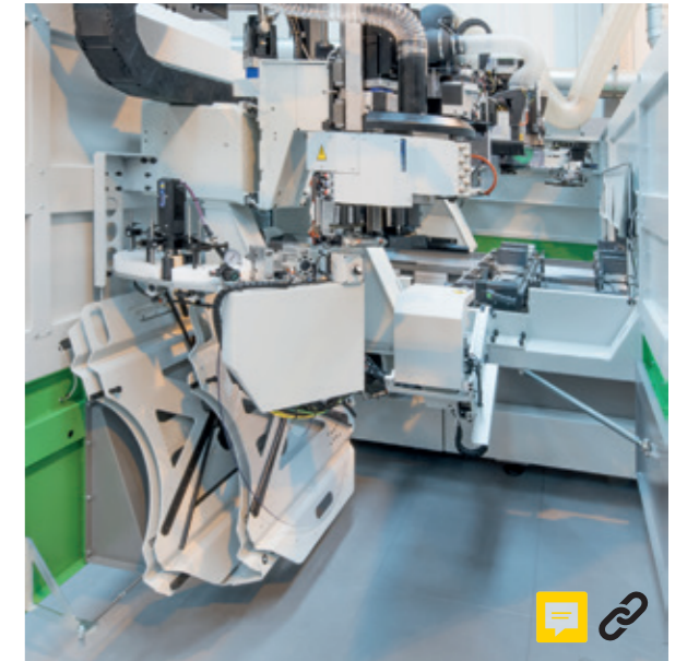
The Rayforce system uses infra-red to create a zero glueline.
