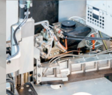
Left: The TM20 hybrid gluepot with the automatic tape feed.
